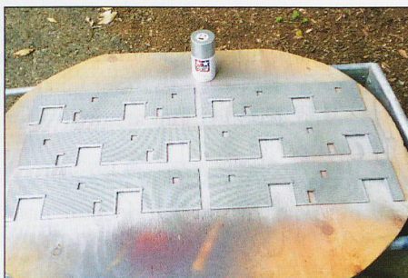
Step 6 - Paint & weather outside for ventilation.
