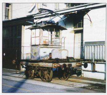
Standard gauge, 4-wheeled, electric shunting loco on Nestlé private siding, adjacent to Chaussée de la Guinguette, Vevey. Works plate reads "Ateliers de Constructions Mecaniques Vevey". Loco appeared to be still operational, note greased buffers, shiny coupling and lack of rust on wheels. 18th September 1989 – photo David Morgan
