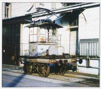
Standard gauge, 4-wheeled, electric shunting loco on Nestlé private siding, adjacent to Chaussée de la Guinguette, Vevey. Works plate reads "Ateliers de Constructions Mecaniques Vevey". Loco appeared to be still operational, note greased buffers, shiny coupling and lack of rust on wheels. 18th September 1989 – photo David Morgan
