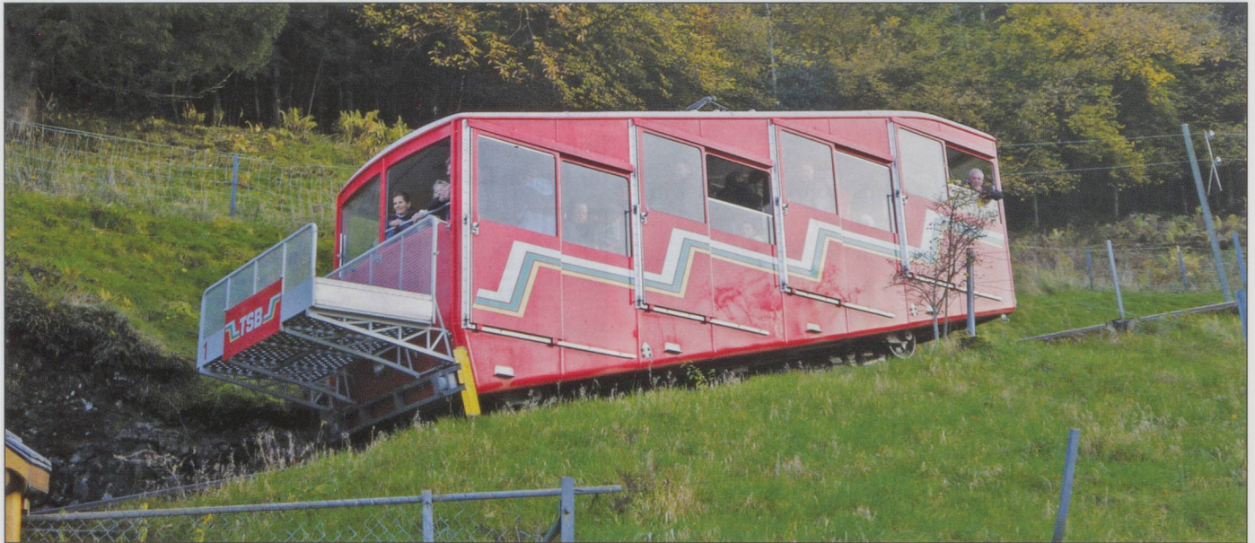
The funicular just outside the bottom station at Treib. Note the luggage rack on the bottom end.
