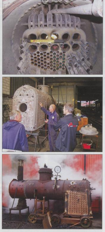
*TOP:* A great view taken inside the boiler. Here we see that the tubes have been cut away leaving only the ends to remove. The inner firebox construction (not original) is held in position at the top by the anchor brackets which allow for expansion movement. The steam pipe mentioned in the main text is the tube positioned top right. This connects the steam cavity in the dome to the regulator.
