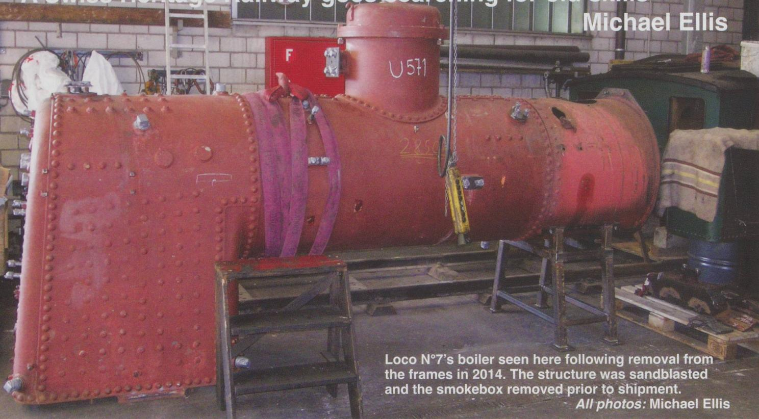
Loco N°7's boiler seen here following removal from the frames in 2014. The structure was sandblasted and the smokebox removed prior to shipment.
