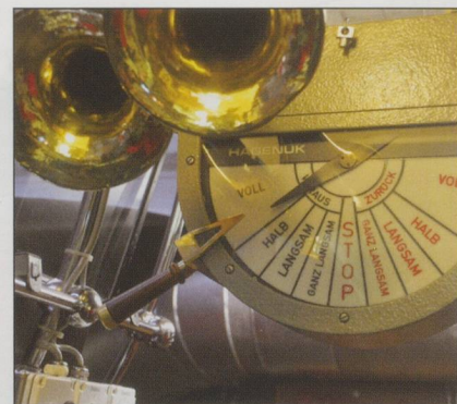
Speaking tube and telegraph to the bridge.
