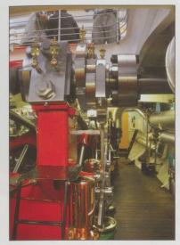
The passageway beside the engine on the starboard side. I was warned to mind the rotating shaft driving the paddle wheels.
