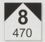
A representation of the gradient board at Mühlenen. The line is shown to rise at 8‰ for 470 m.
