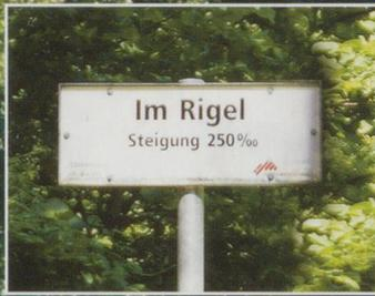
The rack assisted BRB has its own signing system. This shows the start of a 250‰ (1:4) climb.
