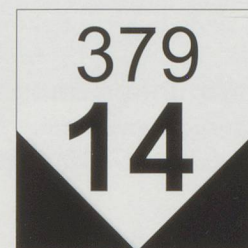
A representation of the gradient board at Le Brassus station. The line falls at 14‰ for 379 m
