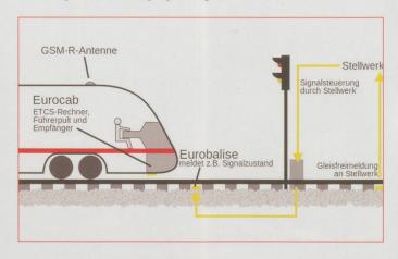
**Level 1** – cab signalling superimposed on the existing signalling system (Stellwerk / Signal Box).
