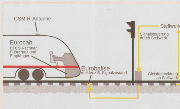
**Level 1** – cab signalling superimposed on the existing signalling system (Stellwerk / Signal Box).
