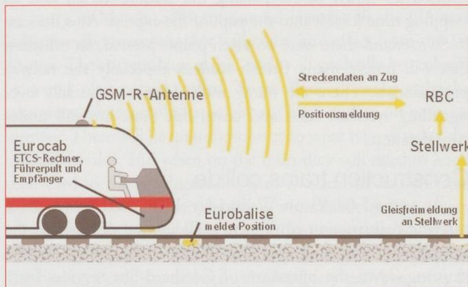
**Level 2** – digital radio based system – all movement authority and signals are displayed in the cab.
