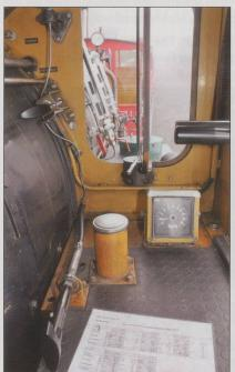
is indicated by a pointer on an almost miniature quadrant. In place of a coal hopper at the back of the cab is the oil tank. While the boiler cladding is just too hot to touch continuously in comfort, the lack of an open firehole door and the large openings in the side of the cab keep the temperature at a comfortable level, though no doubt the low cloud and rain Driver's forward view on the climb.
