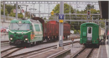
*TOP:* An SBB shunter manoeuvres standard gauge wagons onto metre gauge transporter wheels at Morges.
