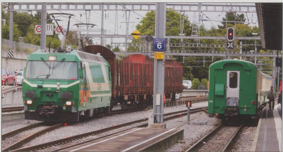
*TOP:* An SBB shunter manoeuvres standard gauge wagons onto metre gauge transporter wheels at Morges.
