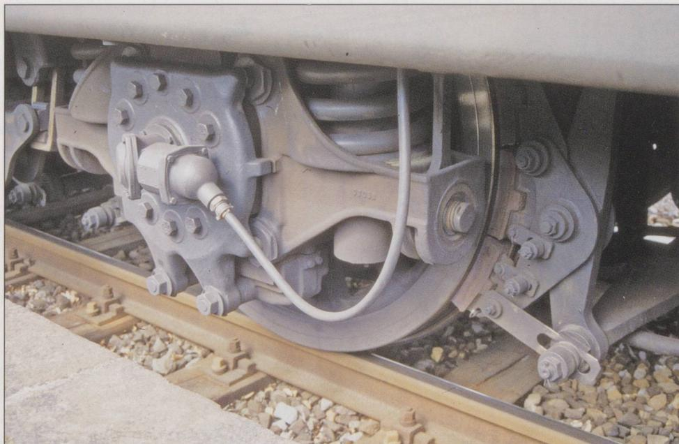
Above: Axle box with speedometer drive, showing the coil springs between axle box and bogie. The lower two of the three brake blocks can be seen.
