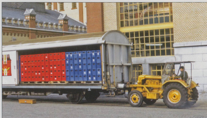
ABOVE: A preserved stationary steam engine. RIGHT: Locomotive shed with ex-SBB 0-6-OT 8481 SLM of 1907 acquired in 1965. BELOW: A wagon being shunted by an adapted road tractor.
