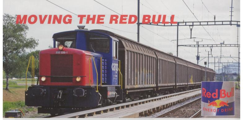
With a brace of RE and four local service movements each hour along the single line, the Tm shunting tractor cannot waste any time when transferring vans to and from Heerbrugg. A standard rake of nine loaded vans hurries through Au SG in the care of Tm 232 226.
