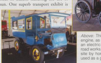
Above: This is not a traction engine, as it first seems, but is an electric light generator for road works. It was pulled to the site by horse power and just used as a generator.
