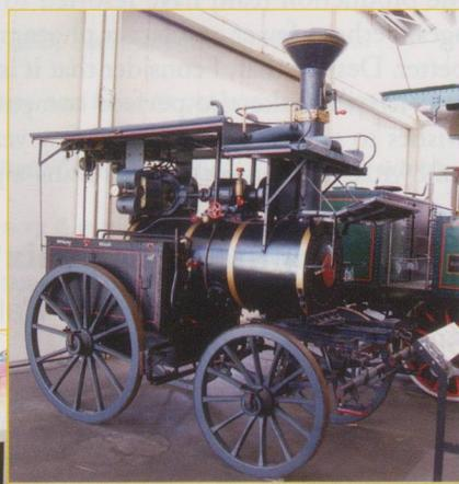
*Above: This is not a traction engine, as it first seems, but is an electric light generator for road works. It was pulled to the site by horse power and just used as a generator.*
