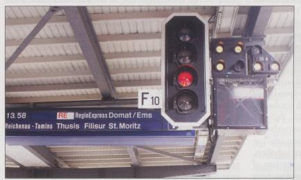
The RhB side of Chur Bahnhof. It may be a bit much to fathom out, but the picture has the following information, from left to right - the train details (for public information); the signal number; the main signal; the brake test (3 white lights show 'test complete and OK'. It will, with green main signal, show when white/green the order to depart); a points signal, two whites showing the setting and a square (blank on the picture) showing restricted freedom (or not) of shunting moves.
