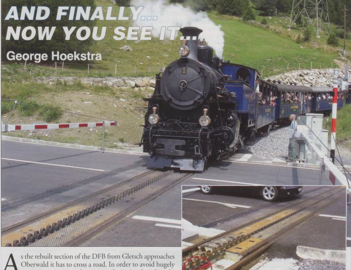
A solution of the DFB from Gletsch approaches Oberwald it has to cross a road. In order to avoid hugely expensive over- or underpasses and associated earthworks this is crossed on the full incline and thus with rack. The rack would rip open every tyre of any vehicle trying to cross it, so a
