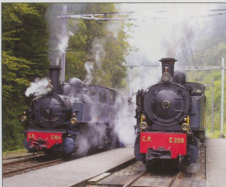
BOTTOM: La Traction Mallets 0-4-4-0T No.164 & 2-4-6-0T No.206 at Combe-Tabeillon, 24/09/08.
