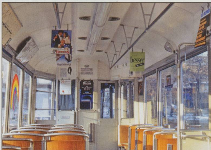
BOTTOM: VBZ 1367 interior. Note the plaques on the bulkhead behind the driver - builders plates in the centre and the full revision history on the left, 01/01/1986.
