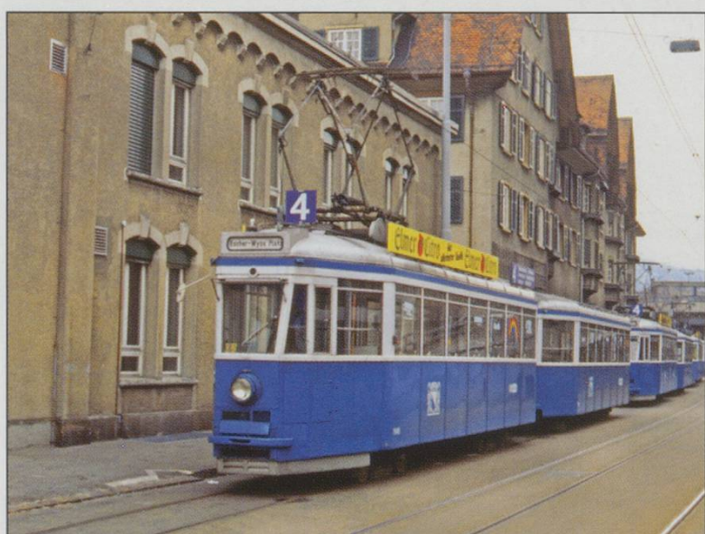
TOP: VBZ "Karpfen" bogie cars 1419+779 at Irchel. Note the odd central window on the leading car designed for an abortive plan to insert an offside door for running in tunnels with central platforms, 08/12/1985.
