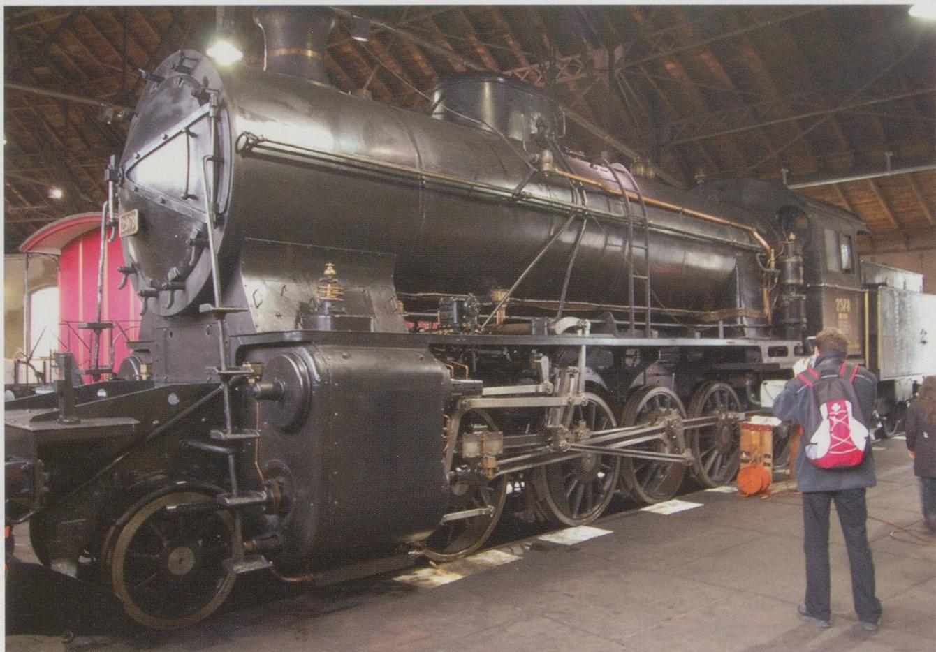
*In the dépôt was the magnificent 2-10-0 "Elephant" No. 2978. When these big machines were put into service, they would not fit into the roundhouse; so two roads were especially extended about 4 metres outwards, just for them.*
