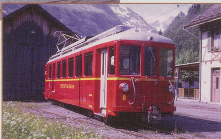
SeTB No. 6 is a CFe 4/4 built by SWS and MFO in 1949 and still at work with the Stern & Hafferl organisation on the Achensee line in Austria. The picture is also taken around 1969 at Elm station by Peter Sutter. The red livery comes from the colour of the regional arms Glarus/Glaris/Glarona with the Saint Fridolin in black on the red ground.
