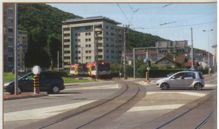
road traffic is halted for train movements. On its route up to Champéry the AOMC gives up street running and becomes a mountain railway as it uses three Strub rack sections to climb 623m to the resort.
