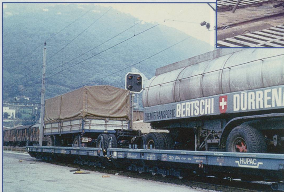
Bertschi drawbar trailer loaded on Wippen wagon
