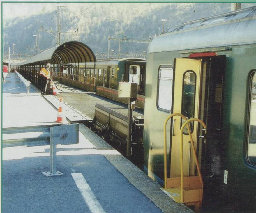
*In Brig, the passenger coach is at the back of the train. For access, the special yellow removable step is needed.*
