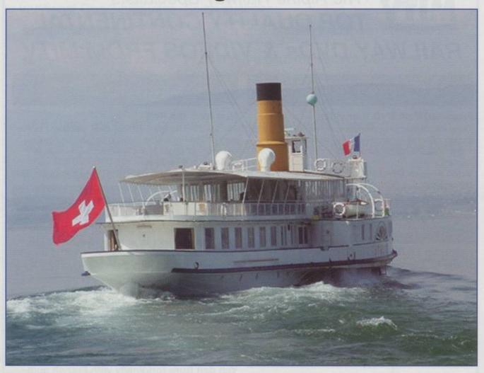
The CGN's ms Italie cruising on Lac Léman. This ship is not a paddle "steamer" as was built, since its paddle wheels are powered by a Sulzer diesel engine. Re-equipping this ship with steam propulsion is now a possibility (April 2005)
