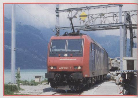
**ABOVE:** 482013 at the discharge site with Vierwaldstattersee in the background. The yellow diamond with a black stripe above the loco denotes the end of the overhead power supply hence the need to use the front pantograph.
