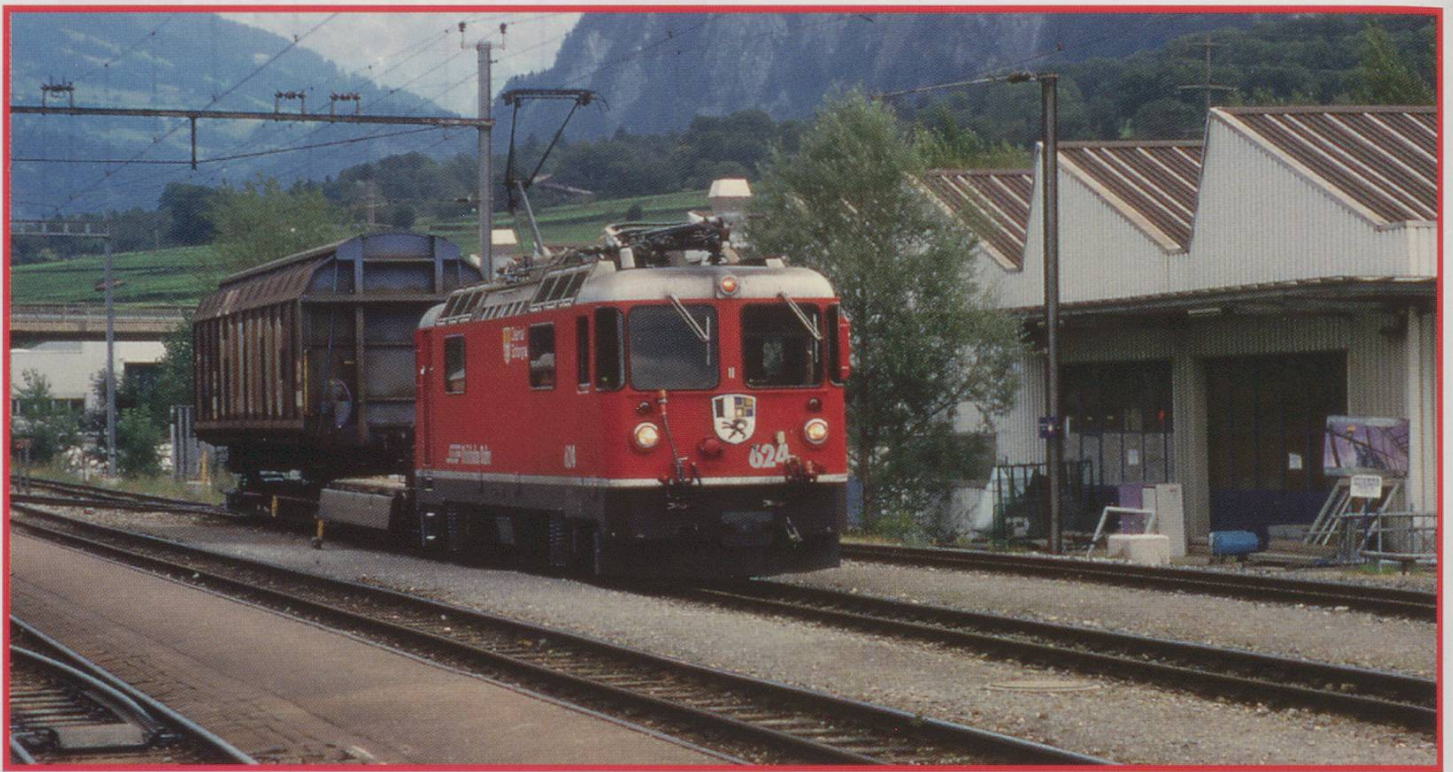
ABOVE; Ge4/ II 624 arrives at Untervaz with a standard gauge truck atop a narrow gauge transporter.
