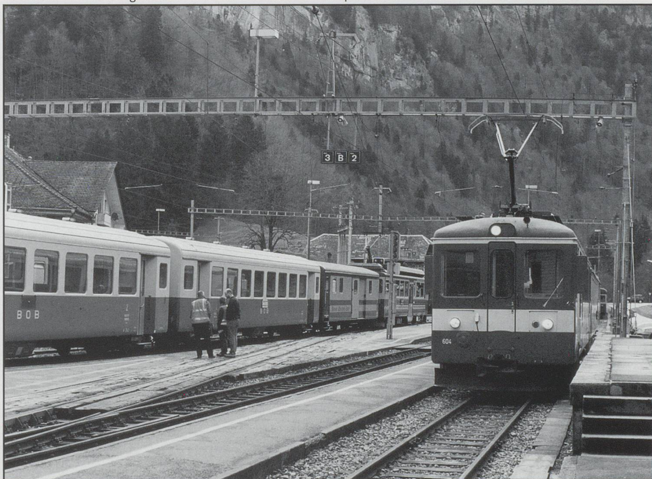
Ex-CJ 604 on test alongside a rake of older stock about to depart for Interlaken with a 1985 motor car in tow.
