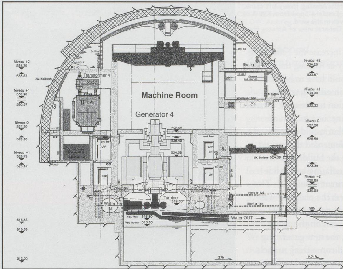
supply is fed to individual oil-cooled 50 MVA transformers fitted to each generator for conversion to 132 KV for feeding via the external switching station to the railway grid system. A diesel generator for emergency supplies is fitted within the cavern. Fire protection for the transformers, generators as well as internal cabling and switches is provided by a Halon gas fire extinguishing system.
