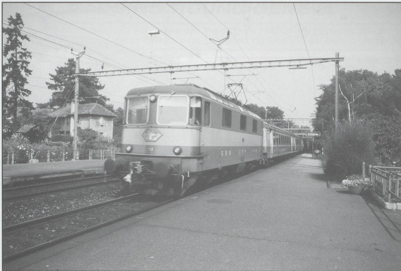
Re4/4 II III13 in Swiss Express livery passes Coppel on a Luzern - Geneva Airport express in September 1982. Note the automatic coupler and the profile of the Mark 3 coaches to allow the bodies to tilt. The locomotive now carries red livery.
