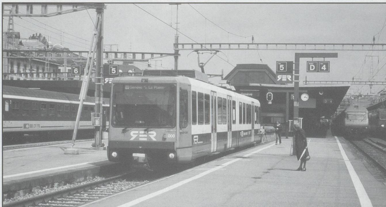
The New Order. Bem 550 000 stands at Geneva Cornavin when working the shuttle service to La Plaine. These low floor units were introduced in 1994, having been built by Ateliers de Constructions Mécaniques at Vevey, with electrical equipment supplied by ASEA Brown Boveri. The yellow doors may not be aesthetically pleasing to all, but they are to assist visually impaired travellers to locate them. The diesel engines are provided to enable them to reach the depot.
