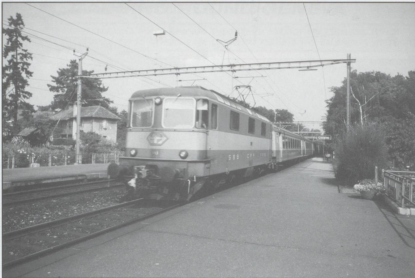
Re4/4<sup>II</sup> III13 in Swiss Express livery passes Coppet on a Luzern - Geneva Airport express in September 1982. Note the automatic coupler and the profile of the Mark 3 coaches to allow the bodies to tilt. The locomotive now carries red livery.
