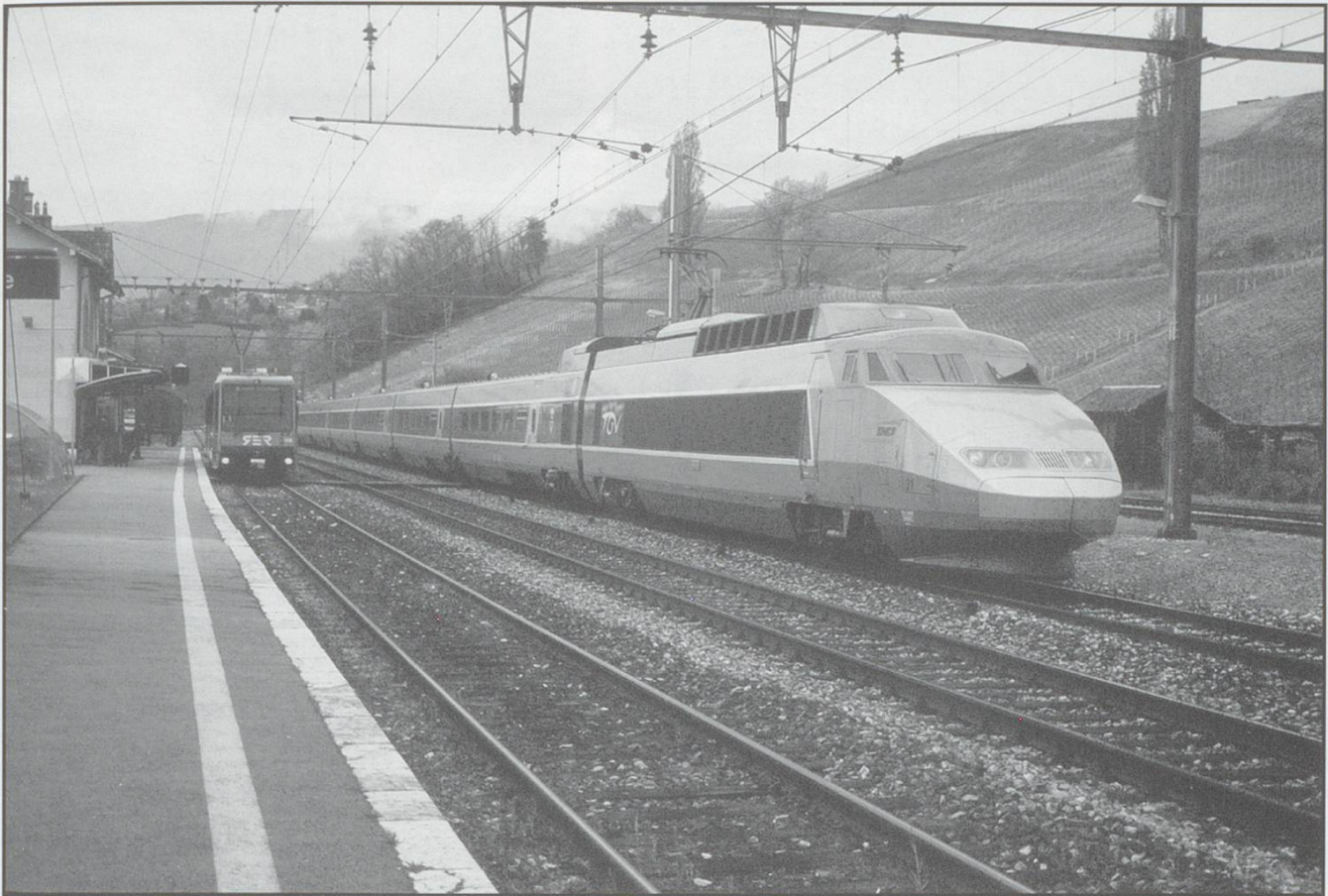
An SNCF TGV unit 31 passes La Plaine on a Paris - Geneva working. Nine units, numbered 100-108, are also equipped to work on the Swiss 15 kV 16 2/3 Hz for through working to Bern and Zürich. Frontier controls are carried out at Geneva. On the left Bern 550 000 waits to take up its next working to Geneva on 29 April 2001.
