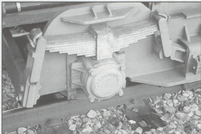
PHOTO 2: The ex-GDR origin of the hoppers manifests itself on the covers of the bearing-boxes: VEB (Volks-Eigenen Betrieb = peoples factory) Achslagerbetrieb (=axle-bearing factory) Stass / Tübingen. One of the new, longer, traverse carrier beams can be seen on the bottom left.
