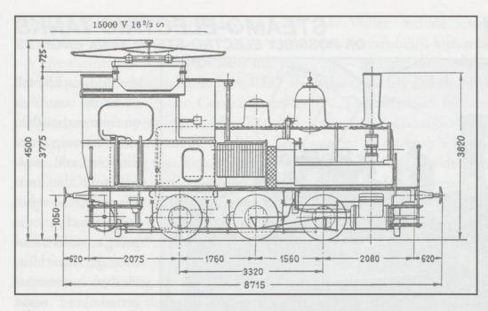
coal fire on the locos, so that they could shunt sidings that were not electrified, but this was kept to a minimum. The weight of all the additional apparatus was 7 tonnes, bringing the gross weight to 42 tonnes. The springs needed strengthening to carry this extra weight.
