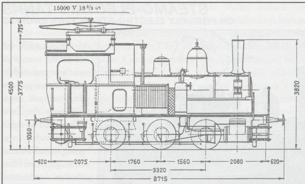
coal fire on the locos, so that they could shunt sidings that were not electrified, but this was kept to a minimum. The weight of all the additional apparatus was 7 tonnes, bringing the gross weight to 42 tonnes. The springs needed strengthening to carry this extra weight.
