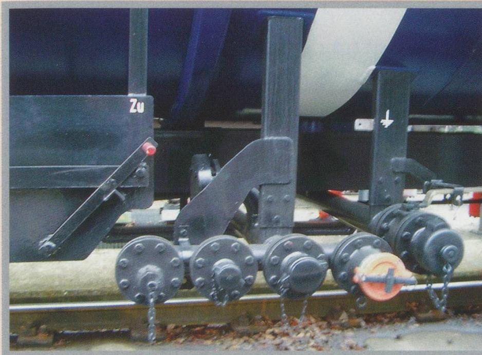
Some of the special connectors at the bottom of the tank car: on the left the connector for the products ("Produktanschluss"), on the right the different connectors for the gas-vapour removal ("Gaspendelanschlüss").
