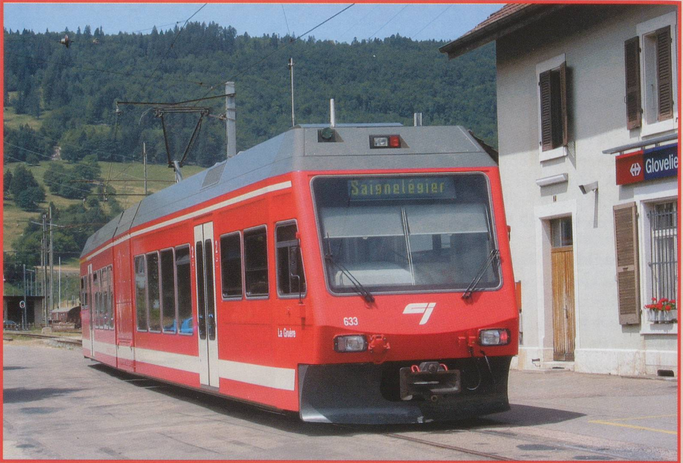
CJ Class BDe 4/4 no. 633 at Glovelier 24th June 2003. One of the new low-floor Stadler units on the Jura system.
