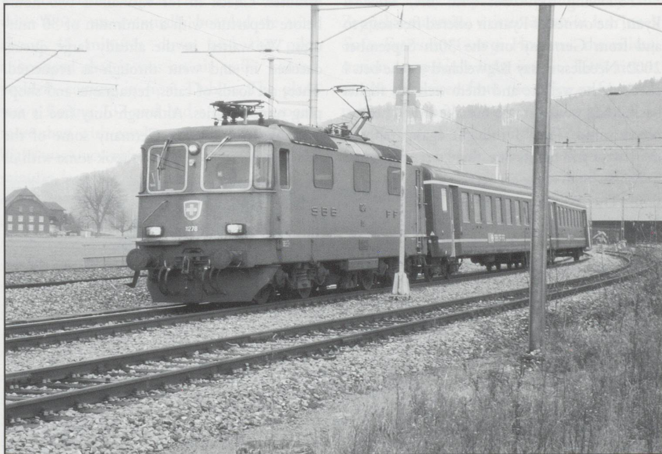
Special Train hauled by 11278 enters sidings at Dagmersellen. The antenna on the loco for the ETCS can be seen, also a TGV style "signal" marker post.
