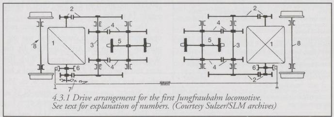
It is easy to understand that the design of steam engines initially had an enormous influence on electric traction vehicles. In 1895 and the following years, the evolution of new drive mechanisms seemed to be problematic, the more so as available electric motors were very large. The locomotives of the Jungfrau and the Gornergrat lines were fitted with 2 motors (1) in my diagram 4.3.1 which ran a toothed wheel transmission (2) on a first backgear (3). The lat-
