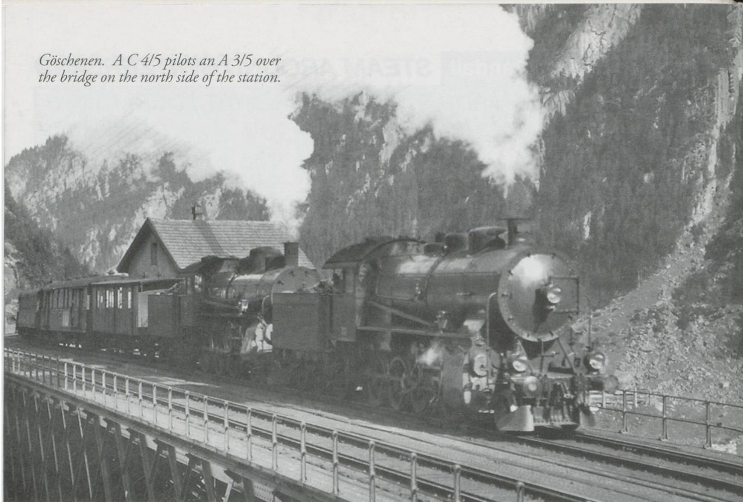
m<sup>2</sup> and the firebox grate 4 m<sup>2</sup> making them the largest of any of the Swiss locomotives.
