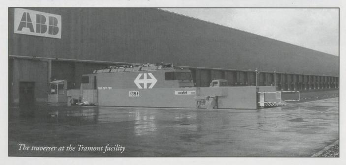
SEPTEMBER 2000 15 via the plant siding and a 300 metre multigauge test track located on the north side. The traverser built by von Roll of Bern has a capacity of up to six axles with a mass of 135 tonnes, and can travel at 100 metres per minute. The use of the traverser removed the need for a heavy lifting crane - capable of carrying the finished locomotive - to be installed in hall one.
