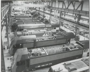
non operational transit bogies. The body containing just pneumatic equipment and pipework is brought from the railway siding to the underpin area where the transit bogie is replaced by support bogies to allow movement around the facility. When this work is complete the body is transported once again via the traverser to its respective bay.
