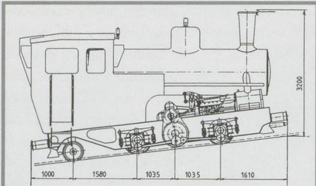
4.1.11 - Outline drawing of the latest steam engine for the BRB. Courtesy SLM
