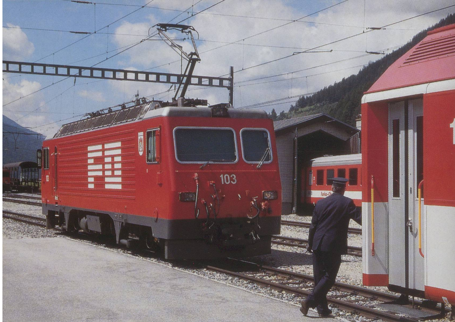
Above: The world's most powerful rack locomotive (see Tooth by Tooth ) FO HGe 4/4 I 103 backs down on to a Glacier Express having dropped off an RhB Restaurant car. Photo: Stuart Frost (see article).
