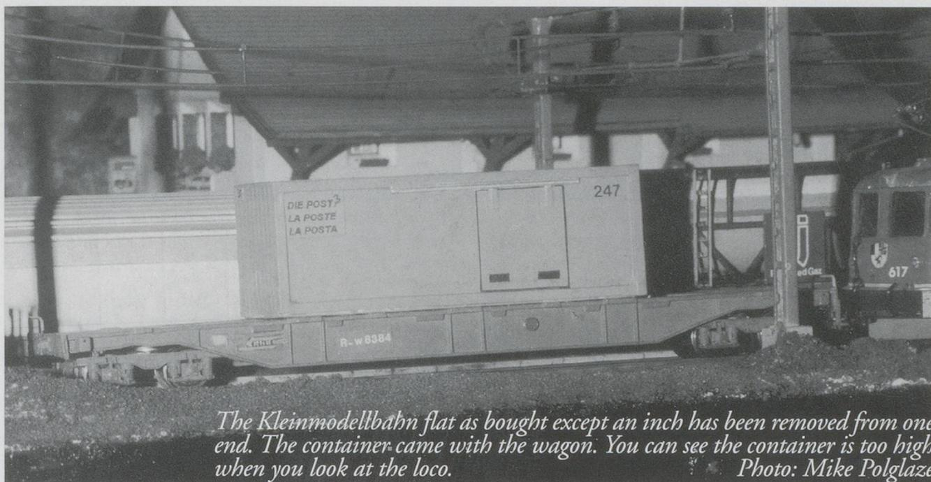
*The Kleinmodellbahn flat as bought except an inch has been removed from one end. The container came with the wagon. You can see the container is too high when you look at the loco.*
