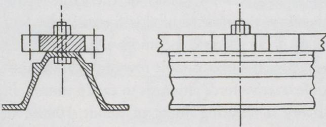
Modern lines are provided with the Von Roll rack which is an improved lamella rack, very sturdy, made for high tooth pressures, easy to manufacture and to lay. In principle it is one lamella of the Abt rack, but heavier and of greater width.
