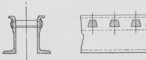
dimensions vary, depending on the tooth pressures, but as far as possible Riggenschbach stuck to a pitch of 100 mm helping in the economical production of the bar. Maintenance is low. One of its drawbacks is the need for higher radius curves than with other systems. (see diagram 3.1)
