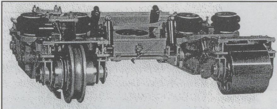
*Drawing 3: The air-suspension bogies. Typical for funicular railways: on the one side a double-flanged wheel; on the other side a roller.*
