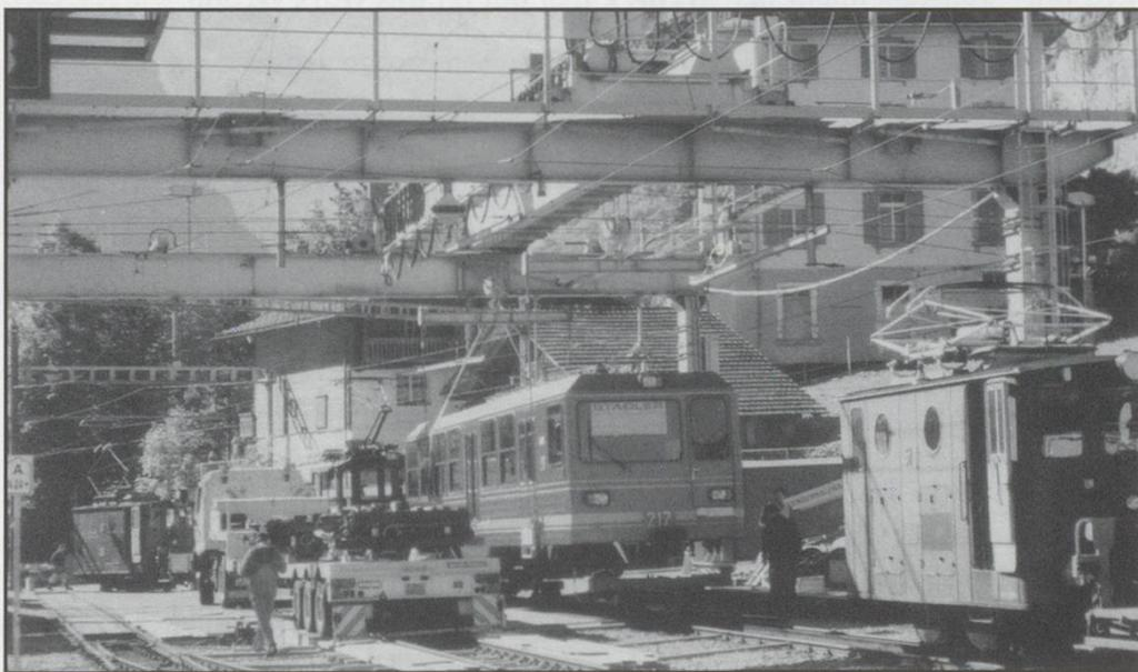
Unit 217 being lowered onto temporary wheels at Lauterbrunnen Station, 17/09/2002.
