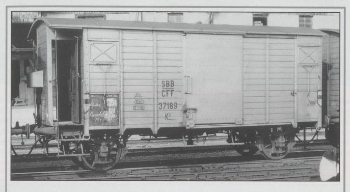
More K<sup>2</sup> vans were built than any other type of goods vehicle in Switzerland. This example, 37189, was photographed at Zürich in 1955. Instead of the usual grey livery, this vehicle had been painted white. Photograph courtesy *Eisenbahn Amateur*.
