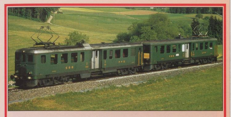
The Be 4/6 railcars were heavy enough to warrant extra carrying axles but, nevertheless, lasted well into the '90's. Two examples, 1607 and 1614, were photographed near Beromünster in May 1992. Although rebuilt, and with only a single pantograph, the livery is still era III green. It can be seen that opposite sides carry the ownership in German/Italian (1607, on the left) and German/ French (1614, on the right). 1614 also carries the yellow/orange warning stripes used on the Seetalbahn.
