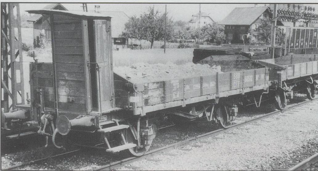
This open wagon dates from 1891 and was 62 years old when it was photographed at Brügg. A feature of the wagon is the semi-open brakesman's cabin. The scant space available and
