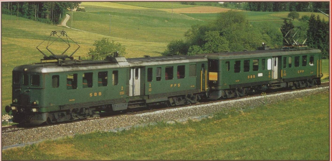
The Be 4/6 railcars were heavy enough to warrant extra carrying axles but, nevertheless, lasted well into the '90's. Two examples, 1607 and 1614, were photographed near Beromünster in May 1992. Although rebuilt, and with only a single pantograph, the livery is still era III green. It can be seen that opposite sides carry the ownership in German/Italian (1607, on the left) and German/ French (1614, on the right). 1614 also carries the yellow/orange warning stripes used on the Seetalbahn.
