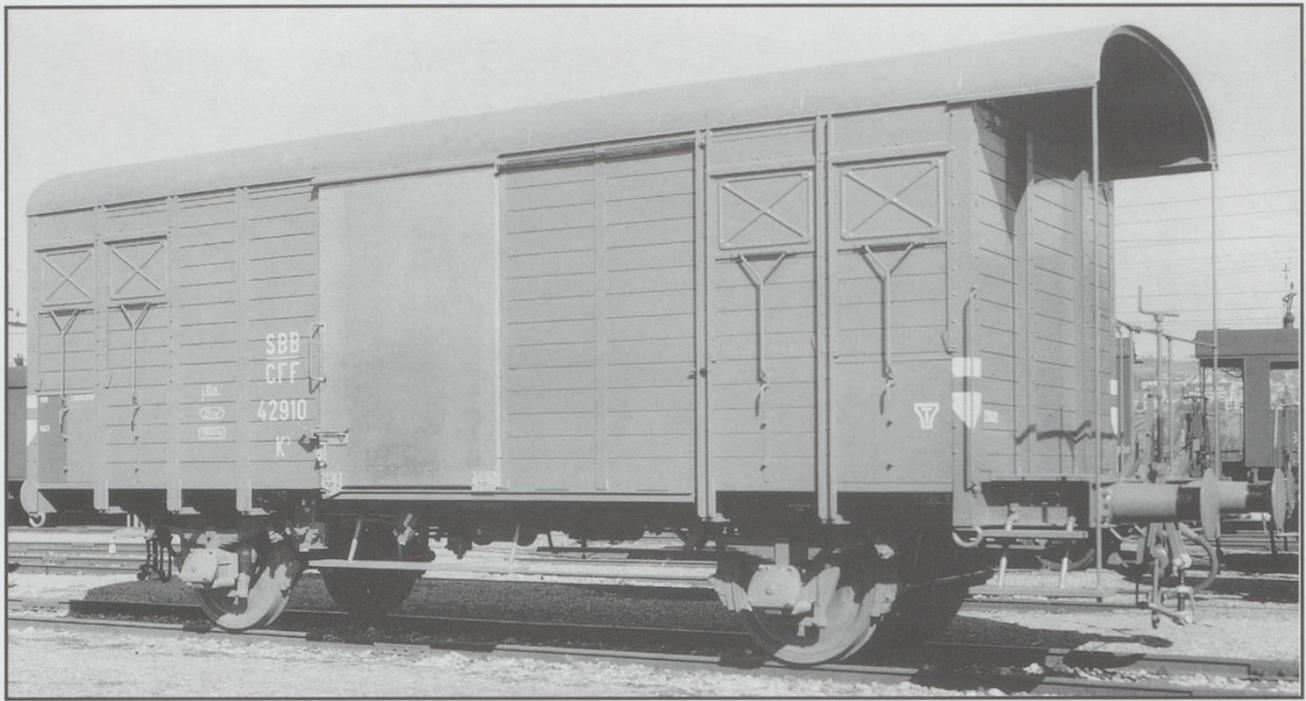
Still a common sight around Switzerland, many of the K3 vans survive as stores vans, etc. This photograph, taken at the end of the 40's, shows the version without a brakesman's cabin. It is not always obvious whether the basic livery of a wagon is grey or brown. The date indicates that, in this case, the wagon is painted grey, with white lettering.
