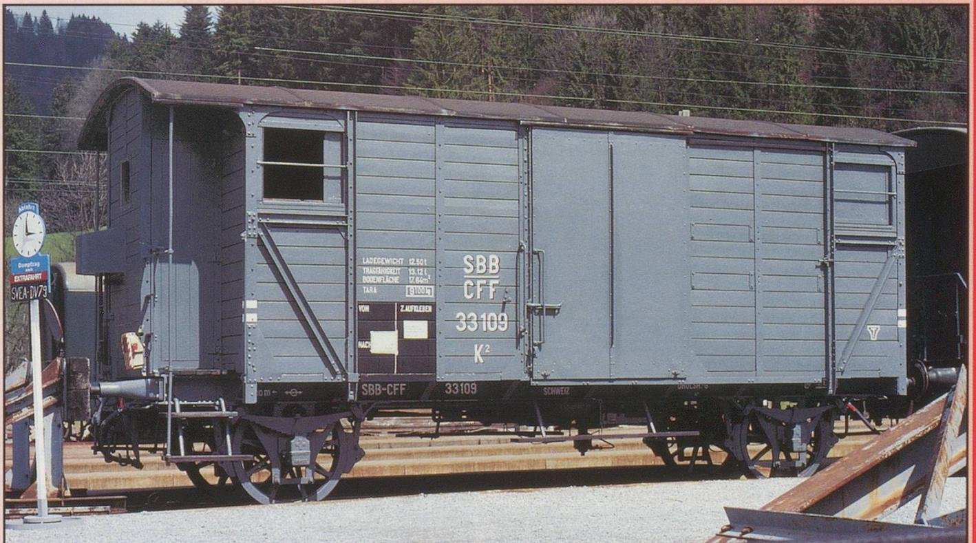
This restored K2 van includes several original features, such as the brakesman's cabin, spoked wheels, open-framed buffers, grease axle boxes and internal sliding ventilation shutters. Also of note is the strengthening ironwork below the ventilators and the curved iron strapping at the top corners of the body. The grey era II livery has shaded principal inscriptions.
