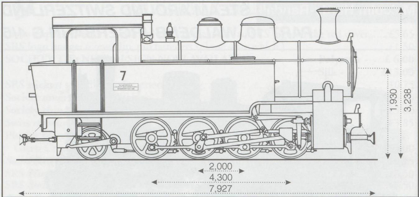
locomotive a fixed driver wheelbase of just 2,000 mm and a total driver wheelbase of 4,300 mm. As all steam locomotives ran down the mountain from Waldenburg to Liestal in the cab forward mode, the carrying axle under the drivers cab was able to provide extra stability on the higher-speed downwards run.
