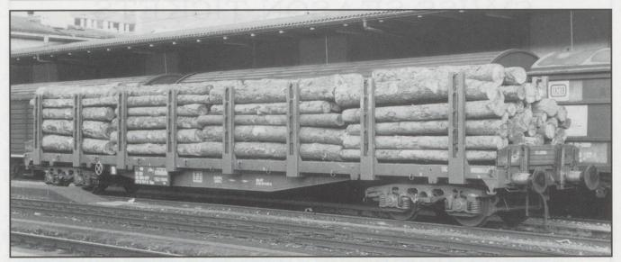
**RAILWAY: SBB CODE:** Sps **TYPE:** 4 axle stanchion, rebuilt from Rs-type WEIGHT: 53 t **COLOUR:** Grey DIMENSIONS: Length 19900mm
