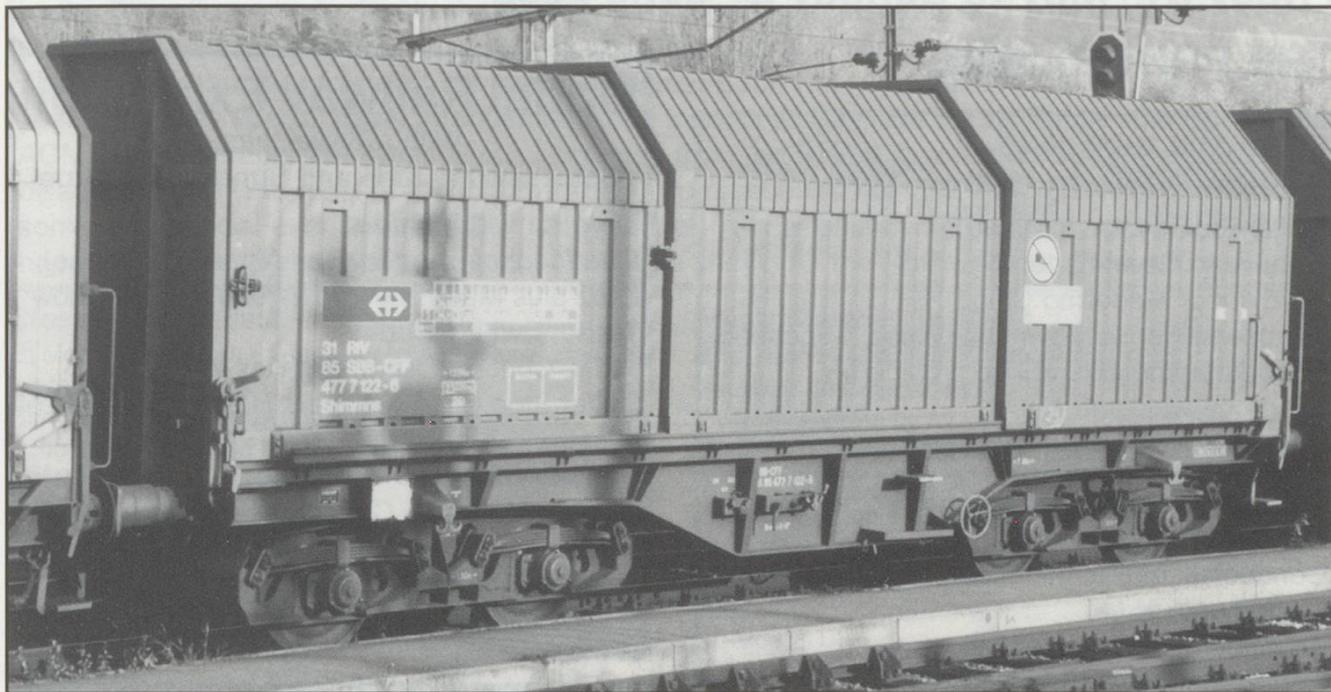
**Railway:** SBB**Code:** Shimmns**No.** 477 7 122-6**Type:** 4 axle steel telescopic cowl wagon**Load:** To carry steel coils under cover**Colour:** Turquoise**Weight:** 59 t**Tare:** 23 t**Dimensions:** Length-12040mm.
