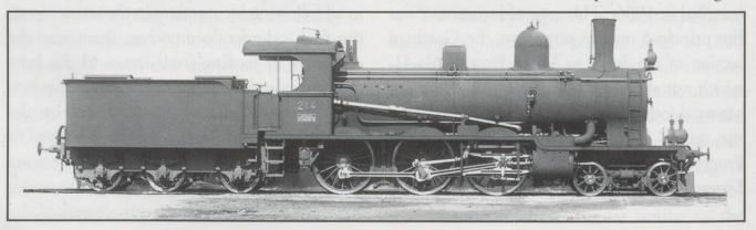
the more efficient Schmidt superheater system. The A 3/5 locomotives remained on express passenger train services until the electric locomotive type Be 4/6 superseded them, and were withdrawn from service in 1926.
